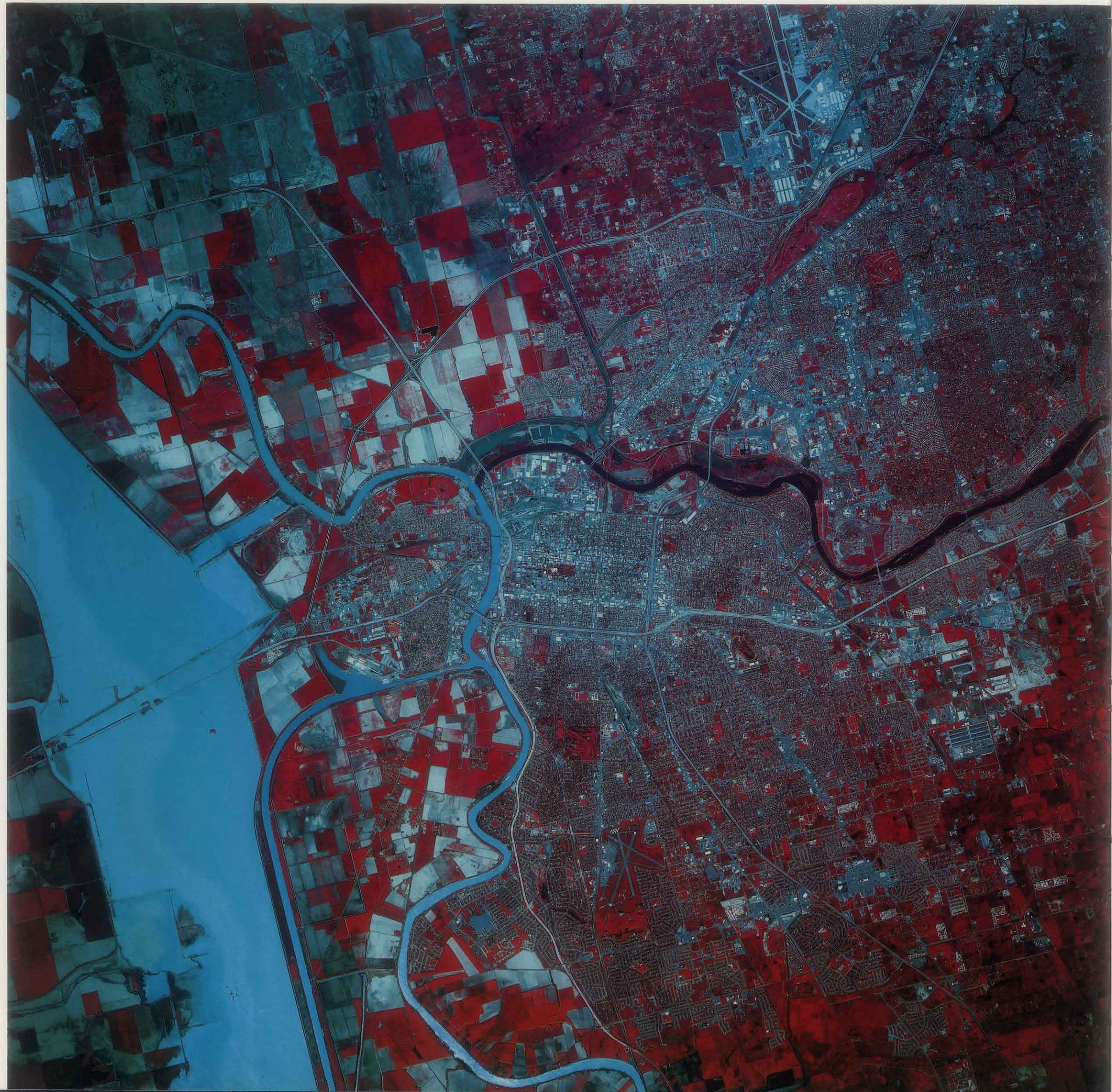
The modern Sacramento Flood Control System in operation during 1975. The Yolo Bypass is shown at the left of the photograph with the Sacramento Ship Channel running next to it. The Sacramento River can be seen entering from the left and curling down through the center. The American River entering at right appears here to have a distinctly darker color than the Sacramento because the American carries less silt.
