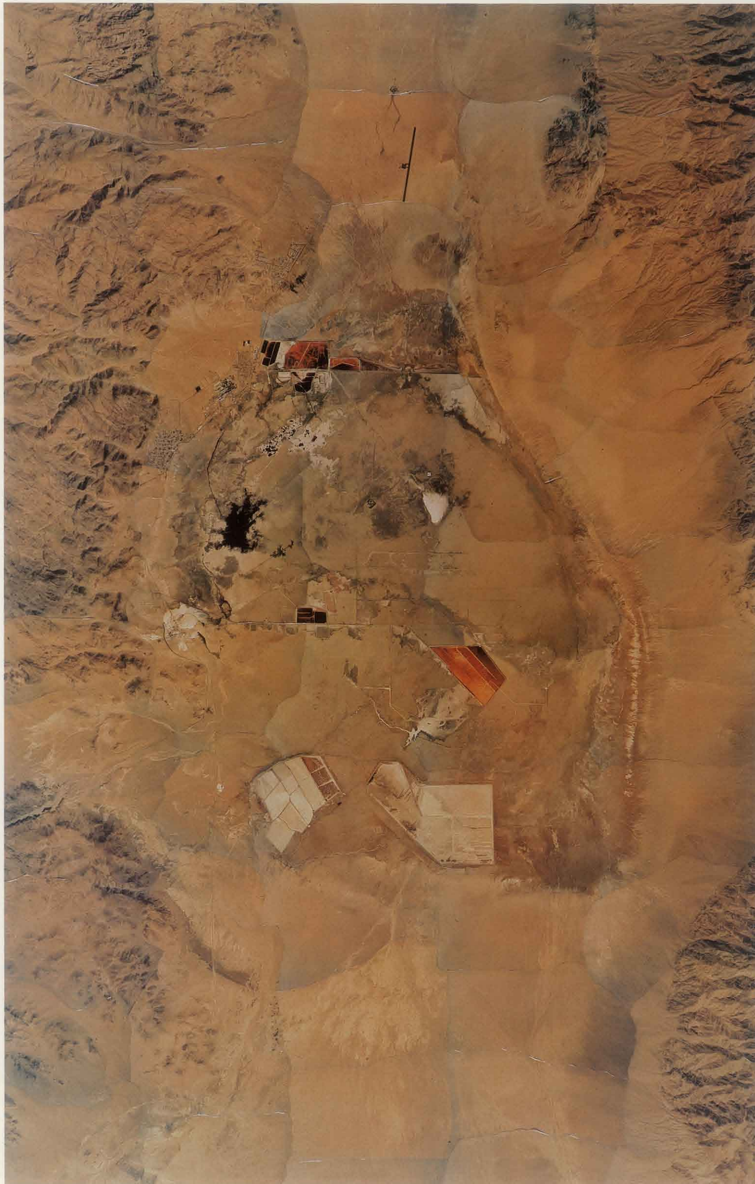
In some areas the disappearance of a pre-existing water source can create economic benefits, as in the case of the mining operation shown here which is extracting commercially valuable salts and chemicals from the dry bed of Searles Lake.
